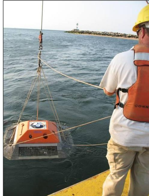
Bottom-mounted current meters were housed in trawl-resistant bottom mounts (TRBM) with Benthos 875 pop-up recovery buoys and Benthos UAT-376 underwater relocation transponders. The subsurface taut-line moorings were deployed with upward looking ADCPs in an Open Seas Inc. SUBS buoy, with tandem ORE CART releases, and an ARGOS relocation beacon.
